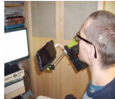
(b) User controlling the computer and the application on a mobile device with his chin
